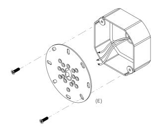
Note: Make sure the supplied Universal Mounting Plate is fastened directly to the junction box. The surface of the junction box should be set back 1/8" or 3mm from the mounting surface. This will ensure the best possible fit for ease of installation and final finish. Note below the correct and incorrect fit for optimum installation.
