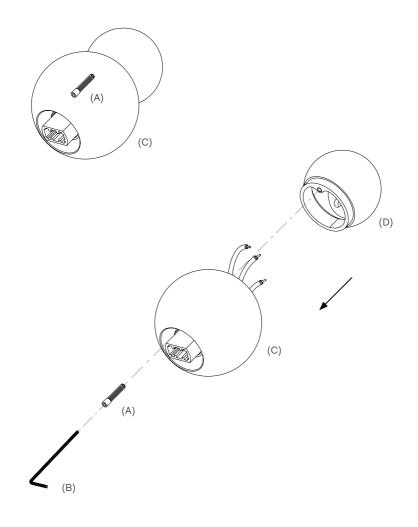
Place the back plate (D) onto the wall, centre it to the mains electrical supply cable and mark two holes to be drilled. Once drilled, insert wall anchors into the holes, ensuring that the area is able to support the entire weight of the fixture (noted on product specification). Screw the back plate onto the wall, making sure it is levelled.
